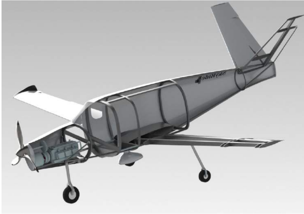
Fig. 9 Internal structure layout of the S270.
