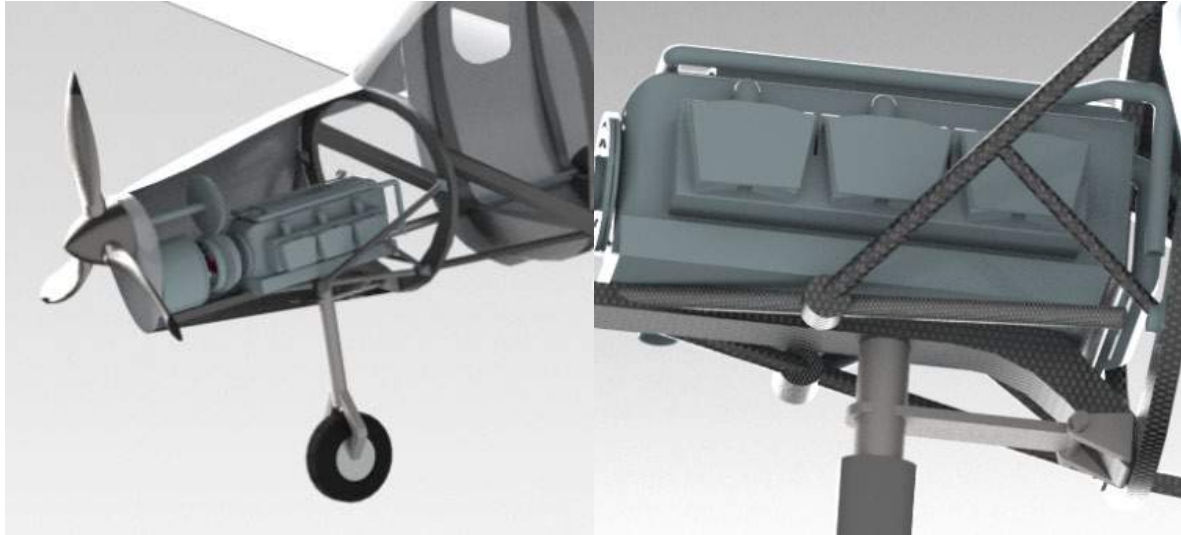
Fig. 51 Engine location in S270 engine bay.
