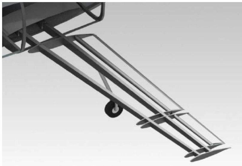
Fig. 58 Wing internal structure layout (skins not shown for clarity).
