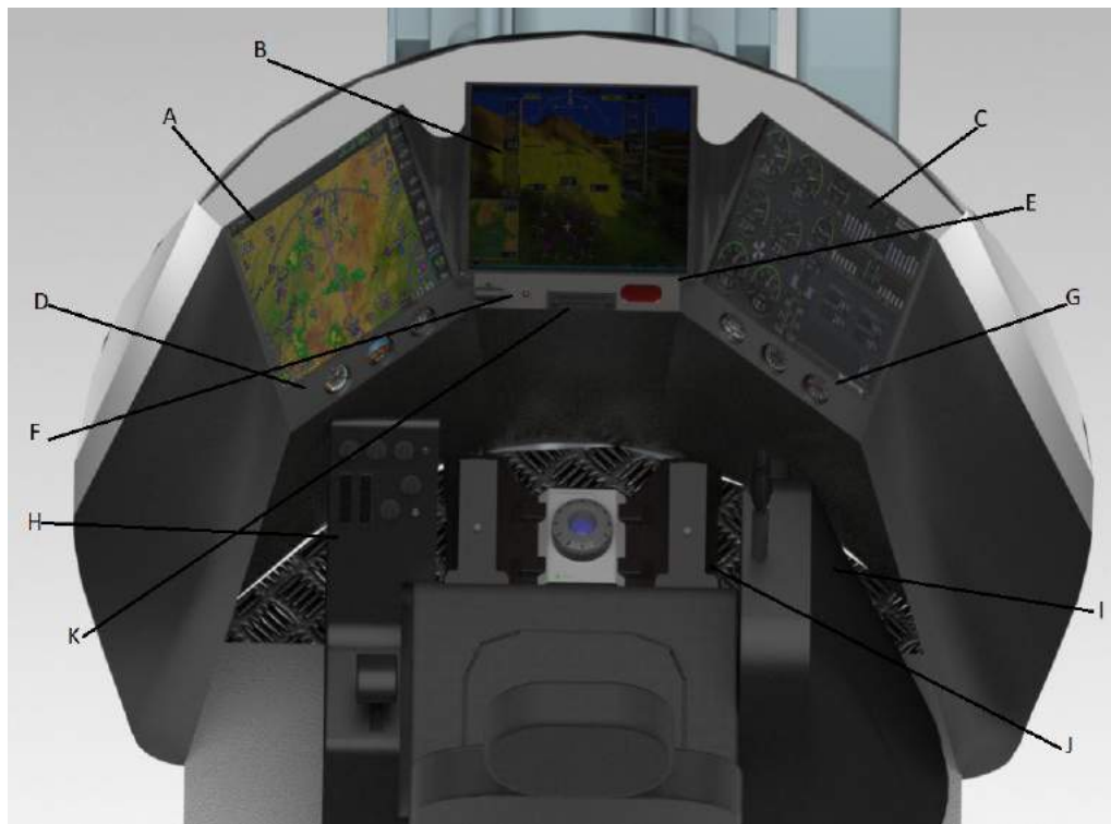
Fig. 79 Labelled cockpit configuration. A – Virtual map display. B – Synthetic vision display. C – Aircraft/mission status and information. D - Airspeed, attitude and altitude indicators. E - Emergency override. F - Parachute release switch. G - Turn co-ordinator, compass and climb rate indicator. H - Secondary Flight Controls. I - Flight Control Stick. J - Rudder Pedals. K - Radio Control Panel
