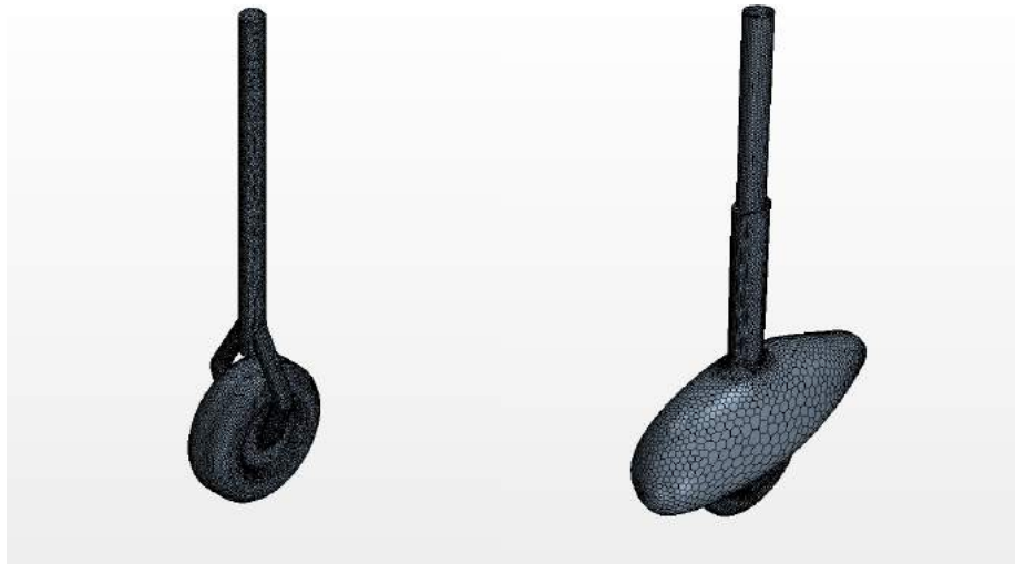
Fig. 26 Candidate landing gear geometries; with and without aerodynamic fairing.
