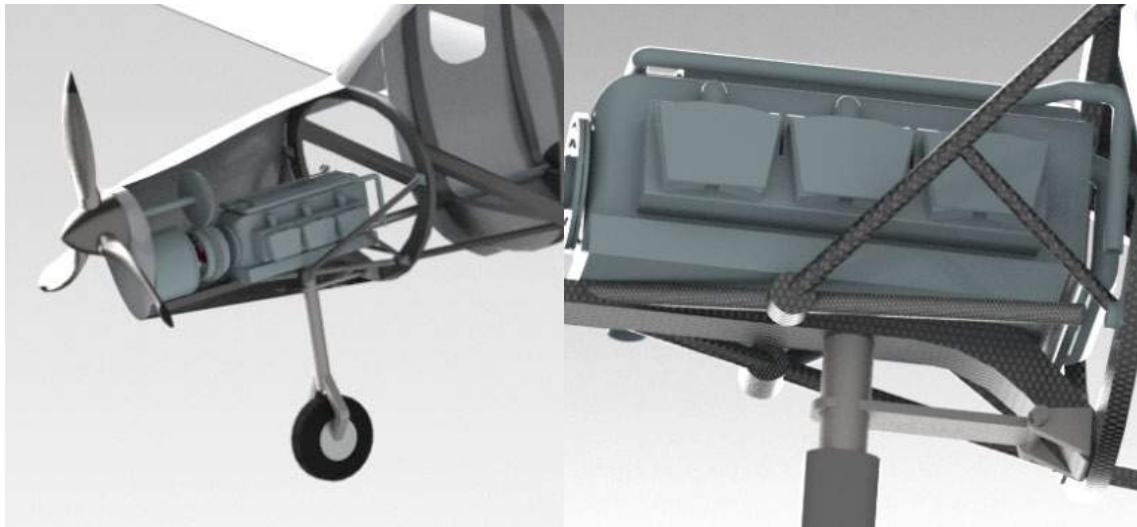
Fig. 78 Landing gear attachment views.
